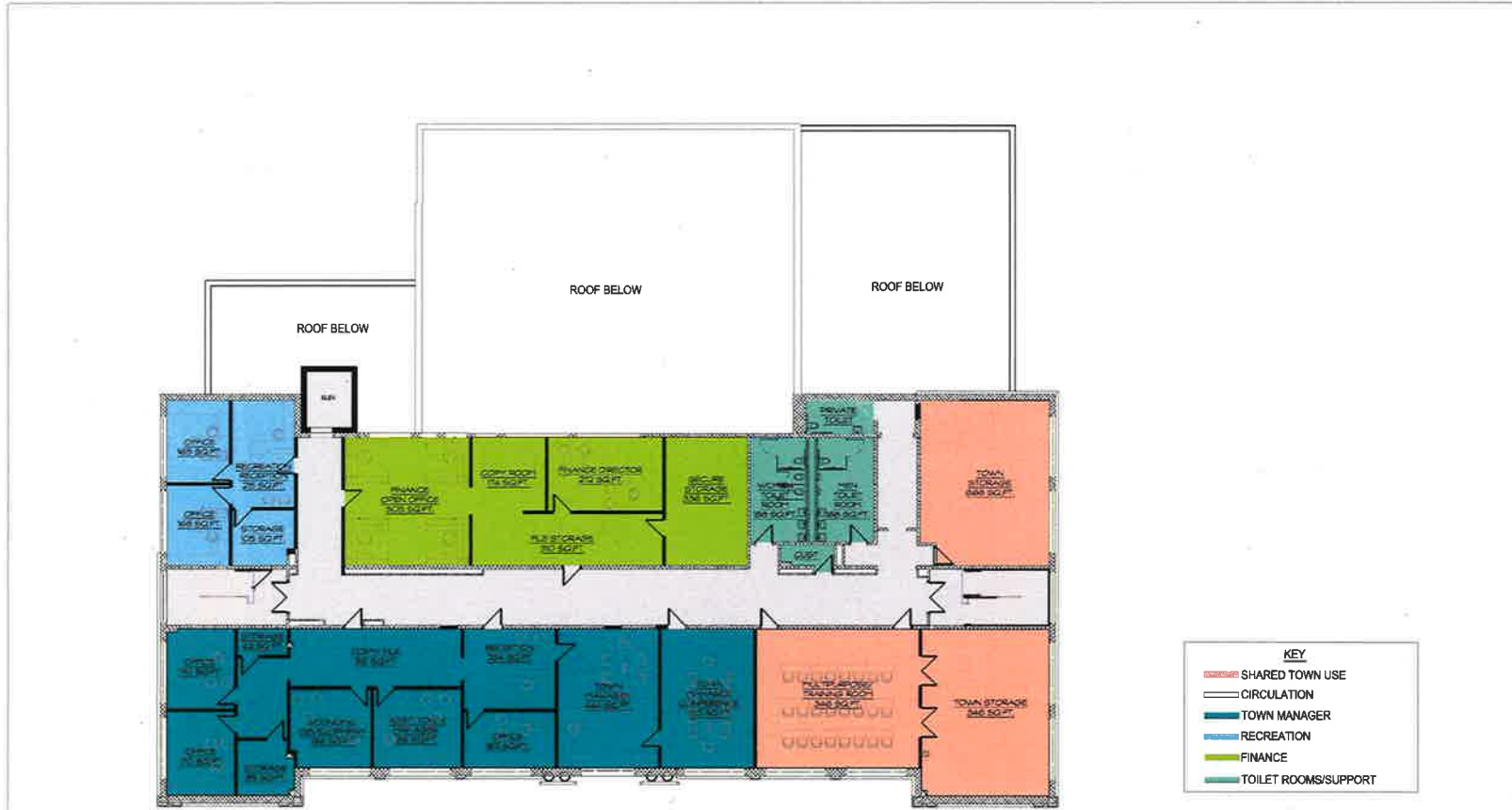
1 UPPER LEVEL FLOOR PLAN SCALE: 1/8" = 1'-0" BUILDING ADDITION: 120 G.S.F. EXISTING AREA TO BE RENOVATED: 10,520 G.S.F. TOTAL MAIN LEVEL AREA: 10,640 G.S.F.
