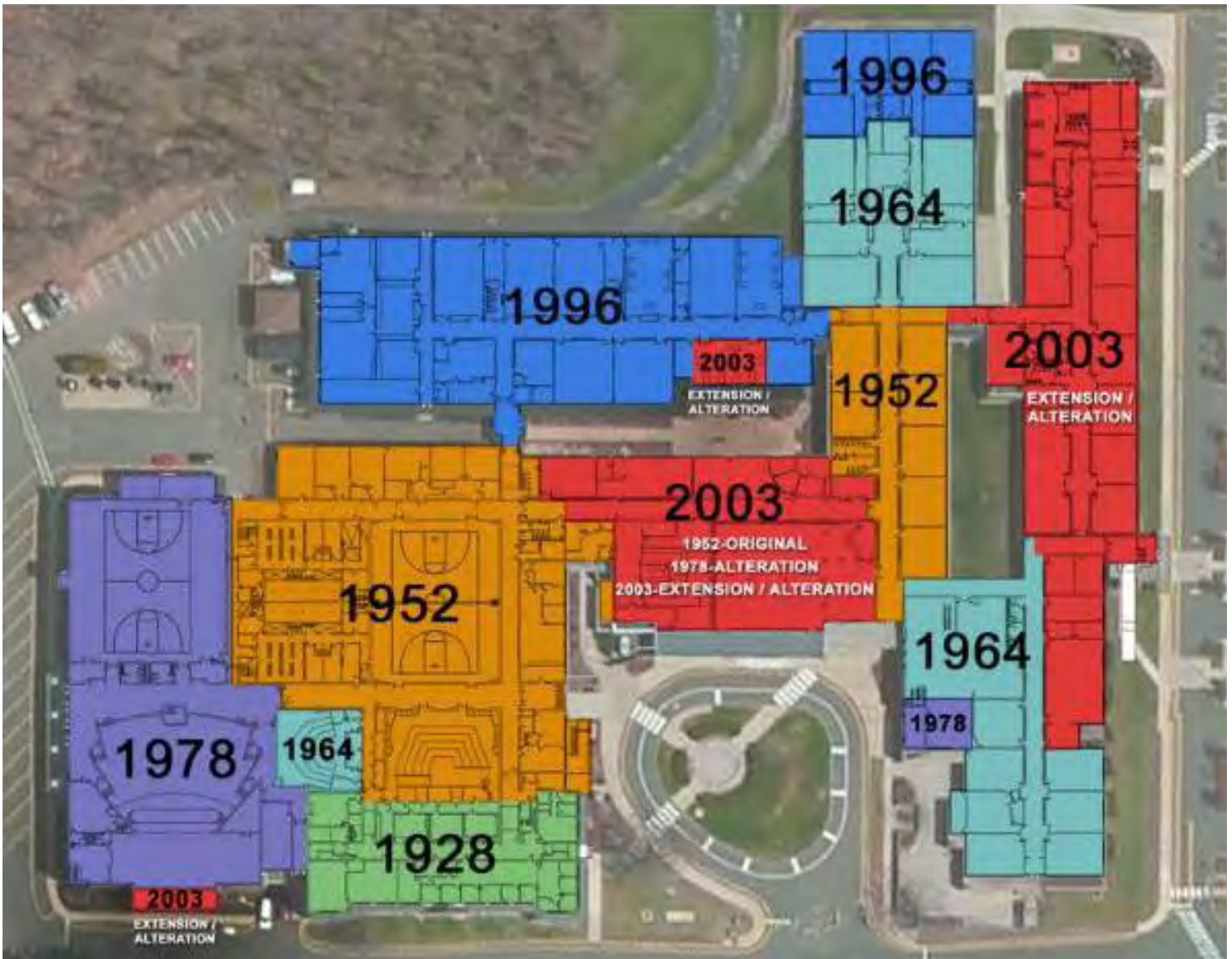
Existing building with vintages of each addition
