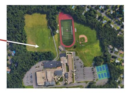
Based on the building area and program, approximately 200 geothermal boreholes at 495 feet depth are required.
